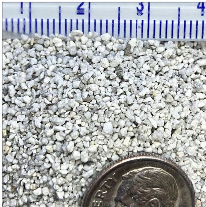
LEFT: Dimension Grit: Monster Bite. RIGHT: Monster Bite used to add surface grip to a non-slip industrial floor coating.
